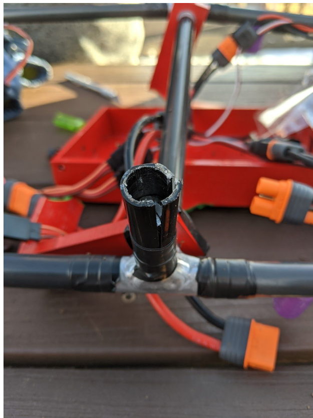
Figure 17: Failed Carbon Fiber Hanger
