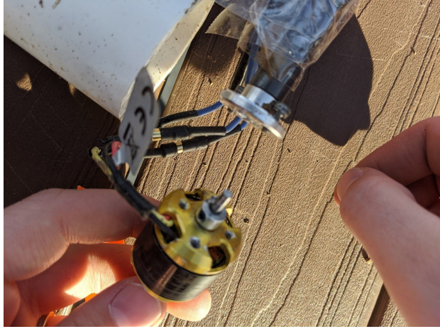
Figure 18: Sheared Motor Mount Screws
