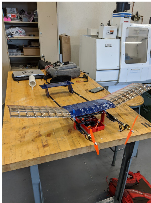
Figure 4: Carbon fiber rods shown in position
